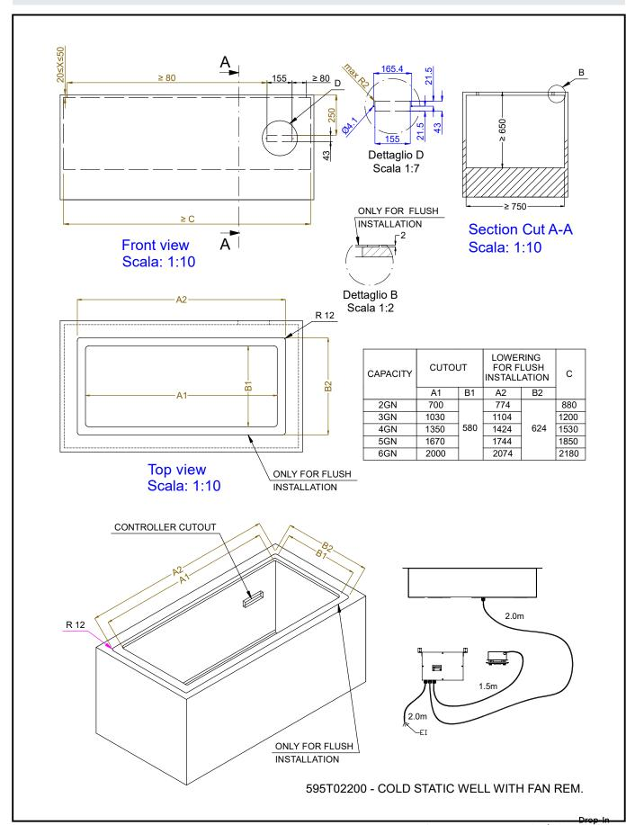
Drop-in remote refrigerated well, static with fan (6 GN container
